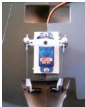
The ailerons are controlled with a center servo and torque rods; a very clean and realistic installation.
