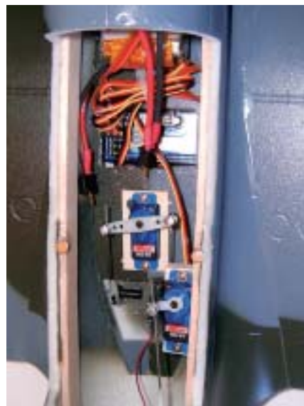
The generous fuselage hatch offers easy access to the radio installation and battery. Note the two rare earth magnets in the fuselage. I added them along with mating magnets in the hatch provide positive attachment with easy removal.
