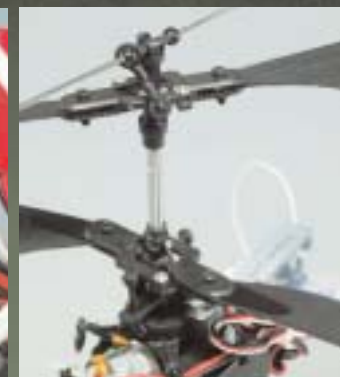
Left: The servos directly drive the swashplate for immediate control. Center: The drive motors are mounted inverted for easy access to the main gears under the fuselage. Right: The swashplate drives the lower rotor while the upper is balanced with a weighted flybar. This design provides exceptional stability in a hover.
