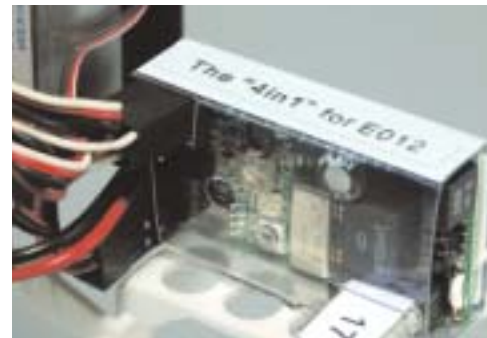
The "4 in 1" unit is the brains of the CoCo Lama, combining the receiver with the motor speed controls, electronic mixer and gyro.
