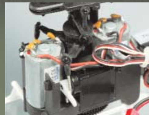
Left: The servos directly drive the swashplate for immediate control. Center: The drive motors are mounted inverted for easy access to the main gears under the fuselage. Right: The swashplate drives the lower rotor while the upper is balanced with a weighted flybar. This design provides exceptional stability in a hover.
