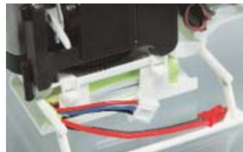
The Li-Poly battery uses a dedicated charge plug to ensure balanced charging and maximum safety.
