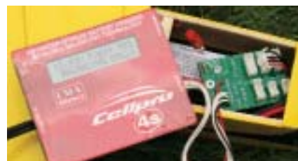
Cellpro charge, from FMA Direct is shown with battery adapter that allows you to charge and balance different brands of batteries.
