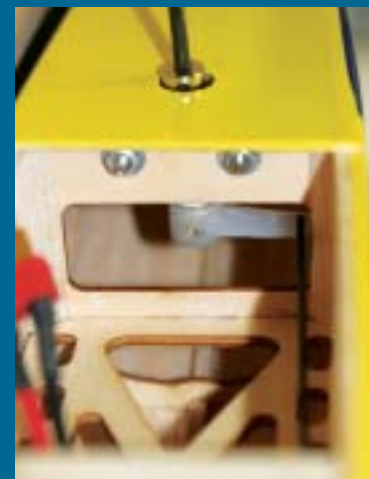
Steerable nose wheel linkage can be seen adjacent to the battery compartment.
