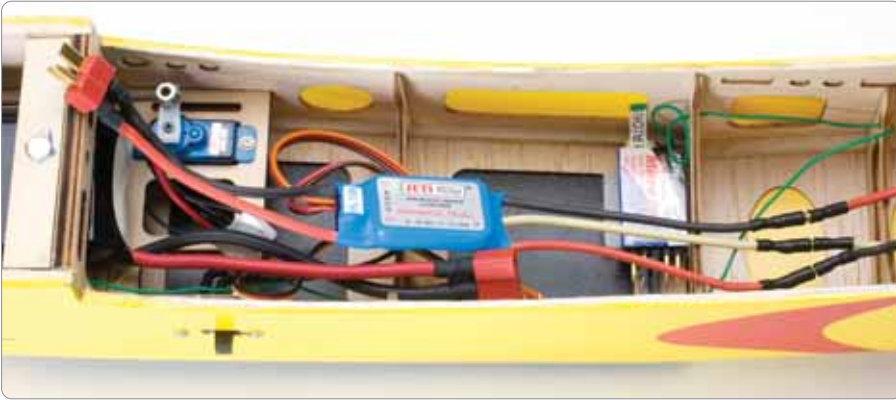
The fuselage has ample room for the nose-gear servo and radio equipment.
