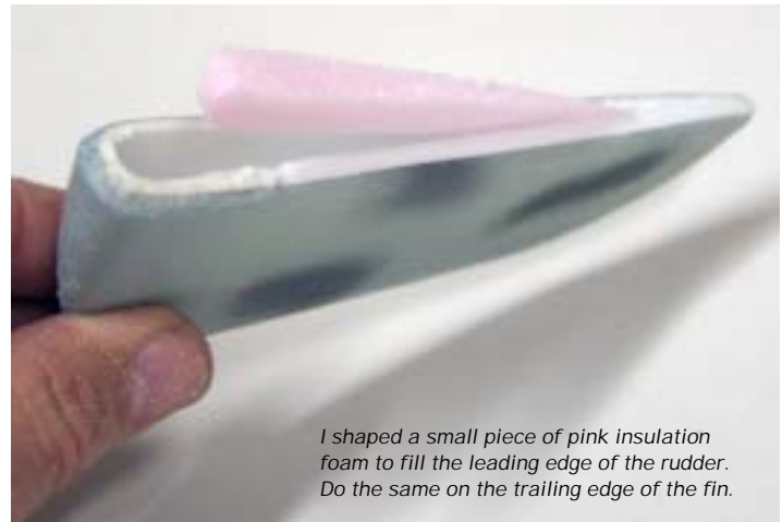
To make the rudder functional, start by cutting it free from the fin.
