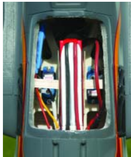
Above left: an old floppy disc makes great hinges for park flyers. A little epoxy securely holds the hinges. Note the GWS control horn. Left: after rounding the leading edge of the rudder, I sanded a matching concave in the fin. Above: the battery fits on edge between the servos. I made a cradle from 1/32-inch balsa to hold the battery. Above right: mounting the motor is simplicity itself: three indentations in the firewall line up the motor right on the thrust line.
