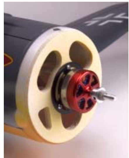
Above left: an old floppy disc makes great hinges for park flyers. A little epoxy securely holds the hinges. Note the GWS control horn. Left: after rounding the leading edge of the rudder, I sanded a matching concave in the fin. Above: the battery fits on edge between the servos. I made a cradle from 1/32-inch balsa to hold the battery. Above right: mounting the motor is simplicity itself: three indentations in the firewall line up the motor right on the thrust line.
