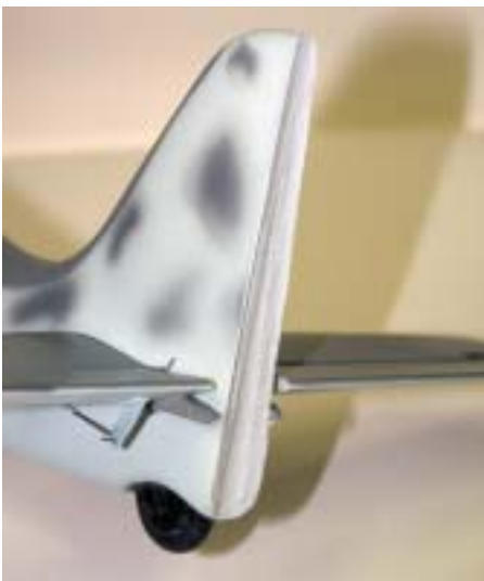
Above left: an old floppy disc makes great hinges for park flyers. A little epoxy securely holds the hinges. Note the GWS control horn. Left: after rounding the leading edge of the rudder, I sanded a matching concave in the fin. Above: the battery fits on edge between the servos. I made a cradle from 1/32-inch balsa to hold the battery. Above right: mounting the motor is simplicity itself: three indentations in the firewall line up the motor right on the thrust line.
