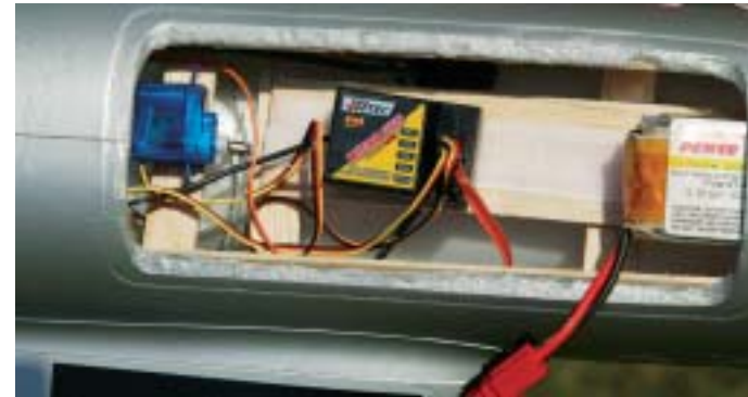
There is plenty of room for the Thunder Power 3S 11.1V 1320mAh Li-Poly battery.
