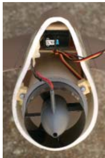
Left: the ducted fan and motor are pre-installed at the factory. The receiver mounts above the engine on a small platform. Right: the recommended battery and aileron servo have ready access under the cockpit.
