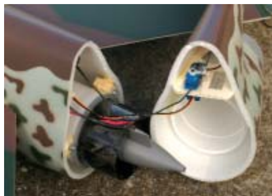
The elevator servo is mounted in the tail cone in a lite ply tray. With the gear in place, the fuse halves are joined with sparing amounts of glue.
