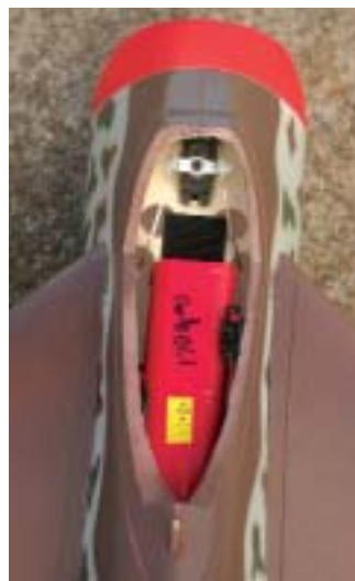
Left: the ducted fan and motor are pre-installed at the factory. The receiver mounts above the engine on a small platform. Right: the recommended battery and aileron servo have ready access under the cockpit.
