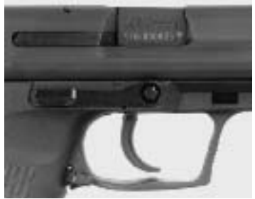
Position of Slide release axle
