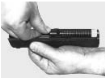
Place recoil spring guide rod on top of the barrel
