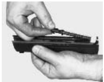
Remove recoil spring, compl.
