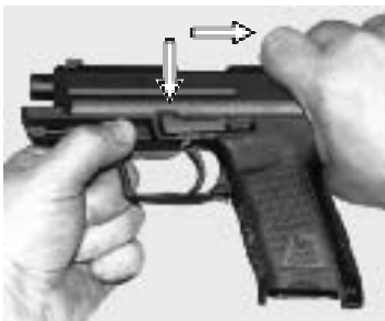
Position of recess with respect to slide release
