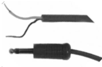
D. Peel back the outside piece of wire surrounding the inner coated wire.
