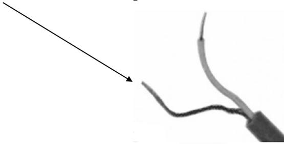
E. With electric tape, tape the peeled back wire to the main cable.
