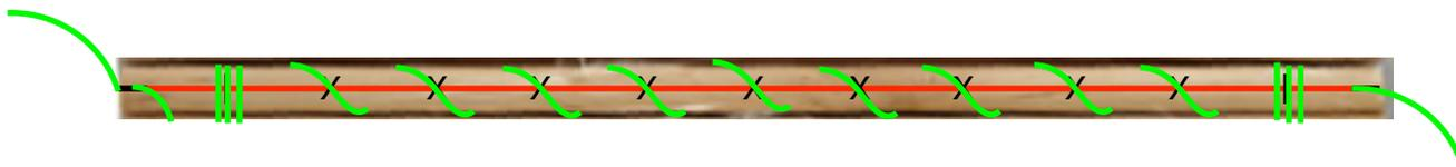
F. Now continue wrapping and once again wrap 3 times around the top hash mark, and then continue wrapping around your dowel until you reach the bottom hash mark. Wrap around this three times once again, and finish by threading through the notch on more time, leaving enough wire coming out of the notch to allow connecting to your alligator clip.
