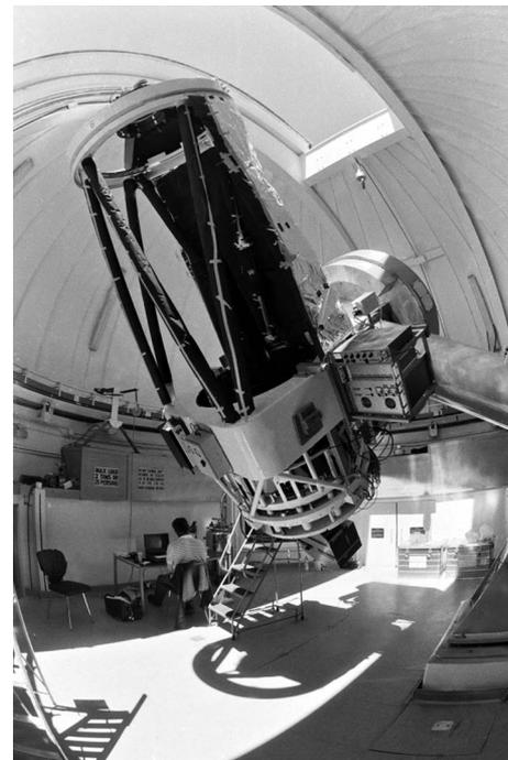
Fig. 1. Multichannel photopolarimeter used for measuring the sky polarization was mounted behind the 1 m Jacobus Kapteyn Telescope at La Palma. As the primary objective of our campaign required daytime observations of Venus down to a Sun separation of 13°, we mounted baffles and screens on the east side of the telescope to shield its primary mirror from direct and singly reflected sunlight [3–5].
