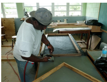
6. Measure trays to fit inside runners (allow 1/4" everywhere), staple on gauze
