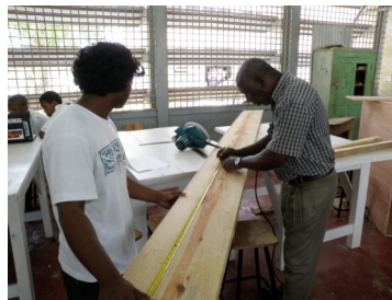
1. Measure pieces of wood to cut from design
