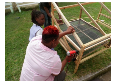
5. Nail in runners, join a 2"*1" with a 1"*1"
