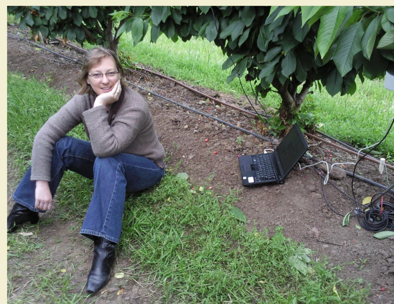
Penny Measham downloading data from a Phyto-monitor data logger recording daily growth patterns of fruit
