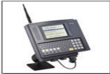
Device used for online Time Recording on Shop Floor. This was integrated to SAP CATS and Project System
