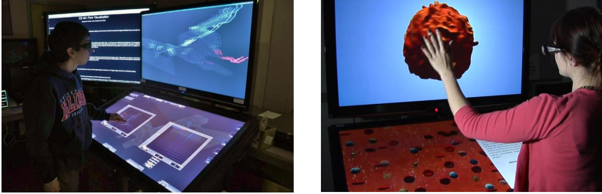
Figure 3. Two examples of OmegaDesk applications. On the left, a flow visualization, showing a 3D map view on the top screen, and multiple configurable 2D plots on the bottom screen. On the right, an educational application displaying blood components.
