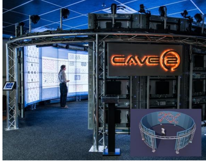
Figure 2. An overview of the CAVE2 Hybrid Reality Environment. CAVE2 is based on a cylindrical setup composed by 18 columns of 4 displays each. This arrangement provides a panoramic view of 320 degrees. Each display pair is driven by a separate computer, for a total of a 36 computer cluster, plus a head node. CAVE2 uses an optical motion tracking system arranged in a circular configuration above the displays
