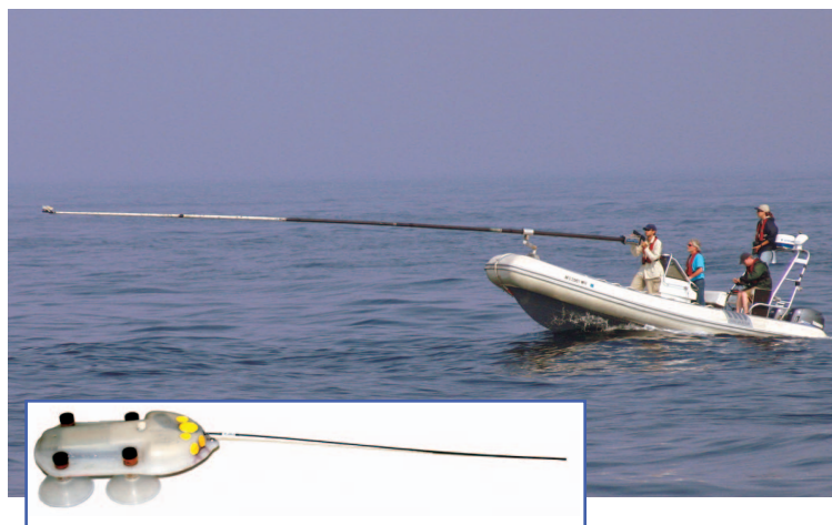
1 The digital recording acoustic tag (DTAG) is attached to a whale using suction cups. Scientists place the DTAG on the whale from an inflatable boat using a 45-foot carbon fiber pole.
