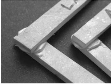
This close-up shows two of the brackets after firing. In each case, an equal and generous puddle of paste was used to make the joint.
