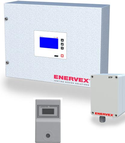
The EBC 35 can be configured either by using the LCD dot display and buttons, or by using the integrated webserver, which also allows remote monitoring and firmware upgrades. Two RS485 ports can be used for Modbus communication, and one expansion board can be used for future hardware upgrades.
