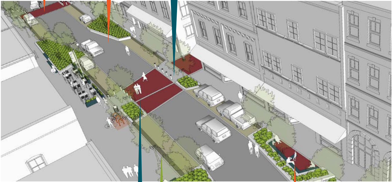
FLEX ZONE DIAGRAM (EXISTING AUTO-CENTRIC STREET REBALANCED AND REPURPOSED TO CREATE A CURBLESS SHARED STREET)
