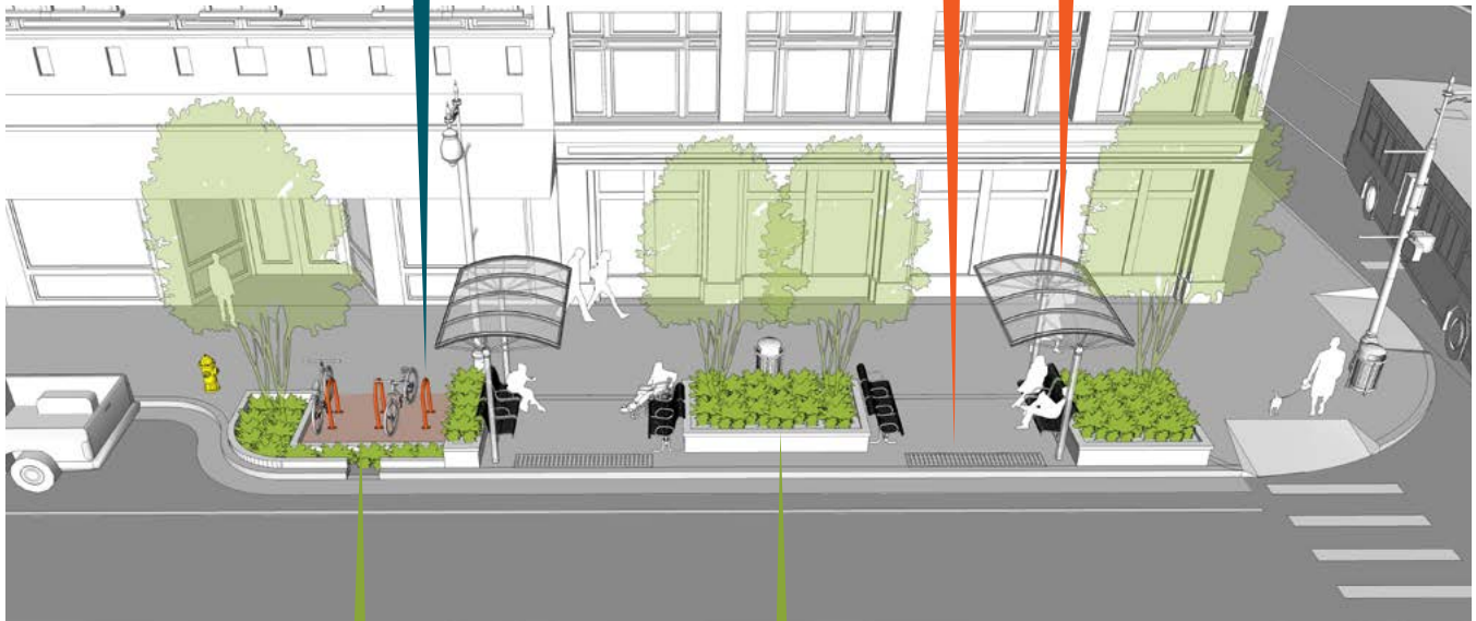
FLEX ZONE DIAGRAM (EXISTING ON-STREET PARKING REPURPOSED TO TRANSIT BULB WITH PEDESTRIAN COMFORT AND TRANSIT EFFICIENCY AS A PRIORITY)
