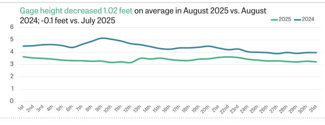
**What is gage height?** Gage height is the distance (or height) of the water surface above the streamgage datum reference point. Gage height is often observed as it relates to landmarks as well as historical data.<sup>2</sup>
