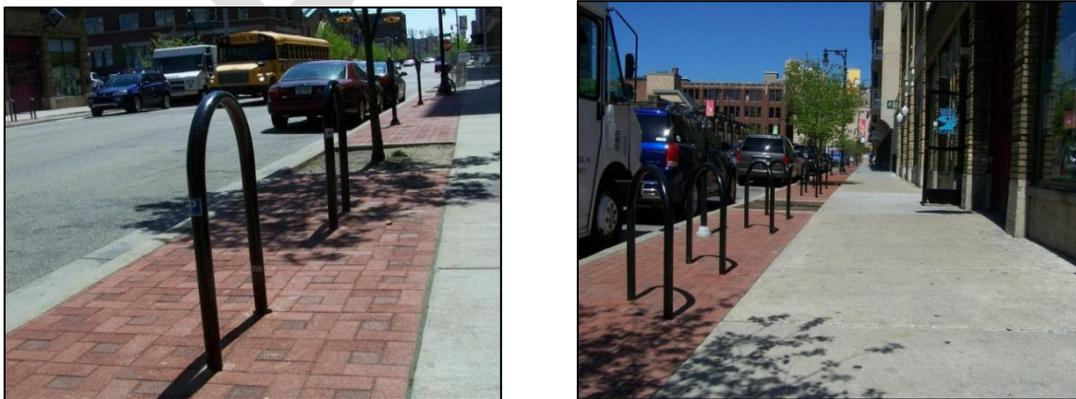
Recently installed U-racks along Commerce Avenue SW: (Right) parallel U-racks from back of curb; (Left) inverted at a 45° U-racks from the back of curb.
