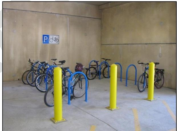
Examples of different types of Class III bicycle parking facilities that are being used parking structures: (Left) a vertical bicycle parking rack in a parking structure in Cincinnati, OH and (Right) U-racks that are being used in a parking structure in Fairfax, VA.
