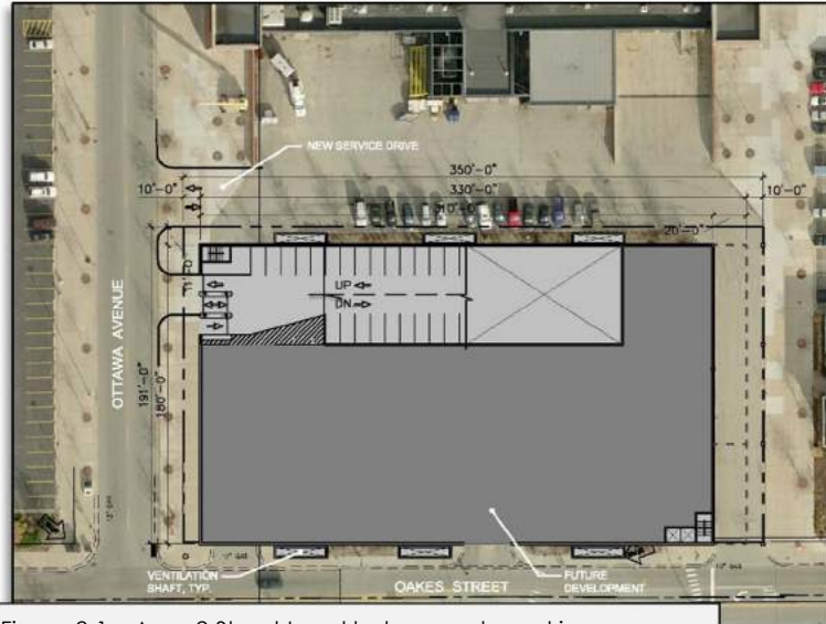
Figure 9.1 – Area 2 Street Level below grade parking access.
