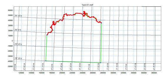
Make sure each open boundary is a separate arc (i.e. has a node at the start and end).
