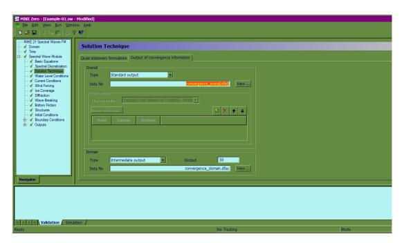
The convergence results are very useful to identify how close to convergence a non-convergent time step is and if the cause of the non-convergence is near the area of interest or if it can be safely disregarded.
