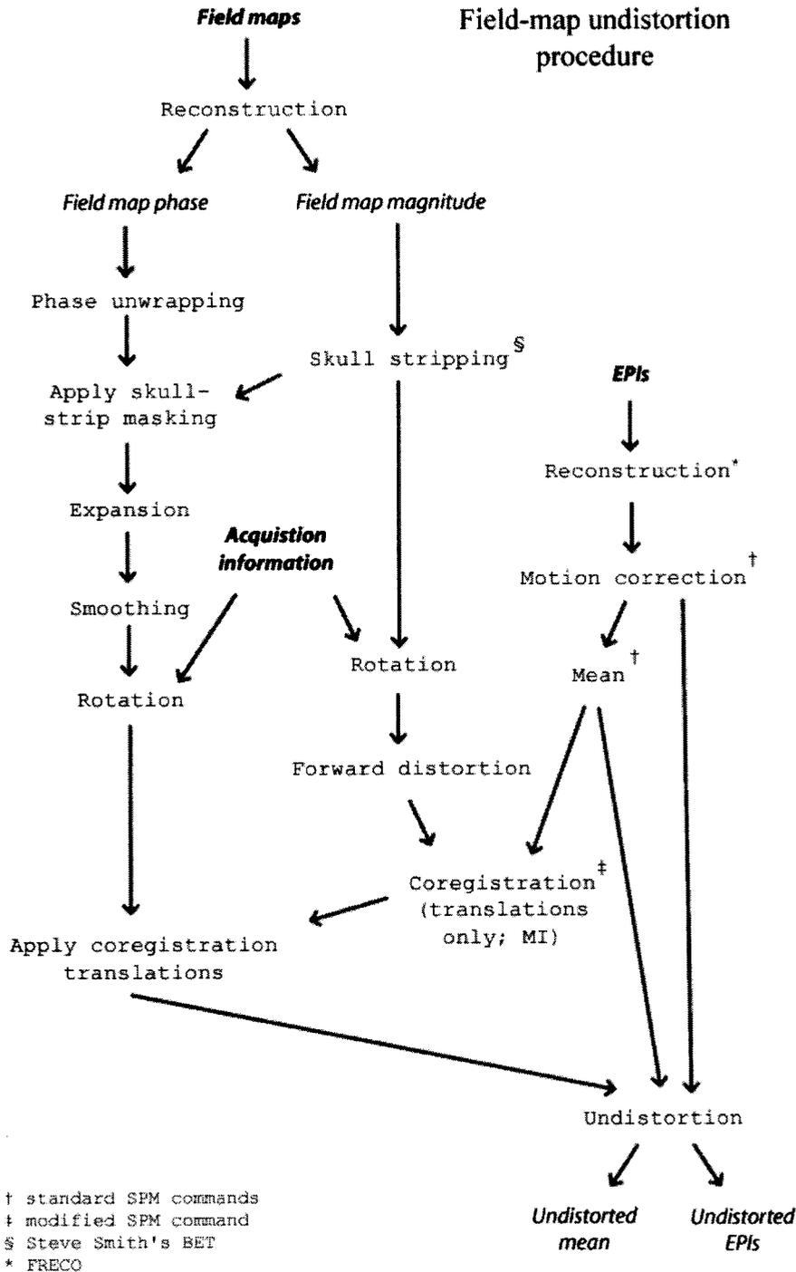
FIG. 1. An overview of the undistortion procedure.
