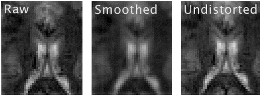
**FIG. 7.** A comparison of the smoothness of the images following smoothing with a filter of 4 mm FWHM and undistortion. A small portion from an axial slice covering the ventricles is shown on a representative subject.
