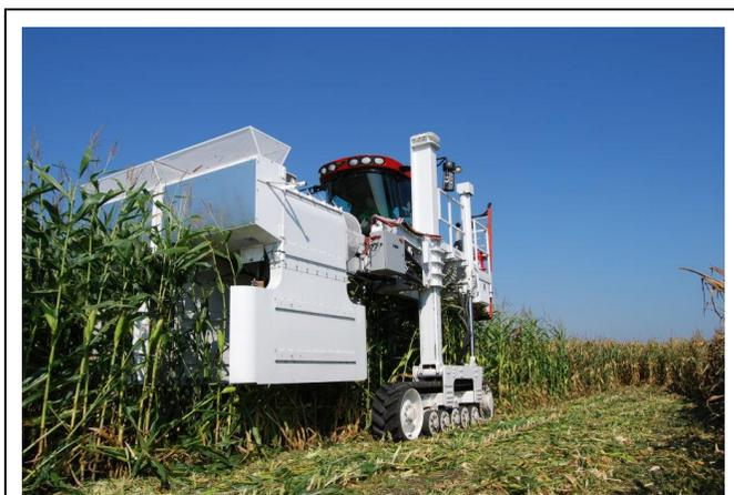
**Figure 4.** “Boreas”, proprietary wind machine, creates winds that can exceed 100 miles per hour to test for brittle snap resistance and standability in corn hybrids.
