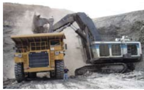
Figure 3: Strip mines use big equipment to remove the overburden then load and haul the coal. OGS coal geologist Brian Cardott stands in front of a large truck and shovel, showing just how massive much of this equipment can be.
