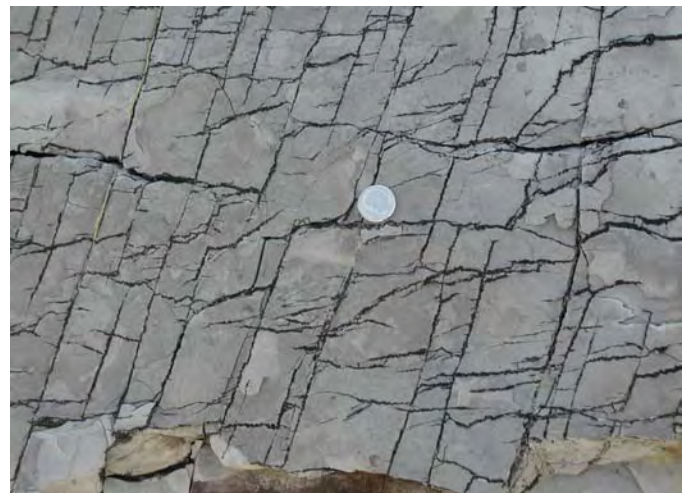
Figure 2. Because of its high silica content, the Woodford Shale is very brittle both in the subsurface and at surface exposures. Show here are fractures filled with dead oil (bitumen). Location; McAlester Cemetery, southern Oklahoma.
