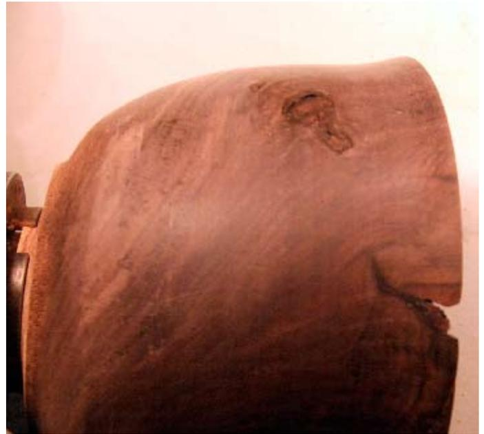
which has been pressing into the bottom tenon. And when I turn on the lathe I see how much out-of-round has happened as the wood dries further and internal tensions are removed. This usually happens, even in dried wood. It all adds to the fascination and challenge of woodturning.
