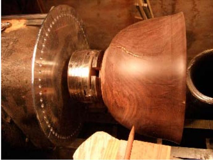
bowl. These were spaced so a shallow flute could be cut, using a 1" diameter router bit. Figure 14 is a close-up. Note that the experimental gold foil filled crack will be essentially wiped out by the fluting. Assuming the crack remains, it will be again filled
