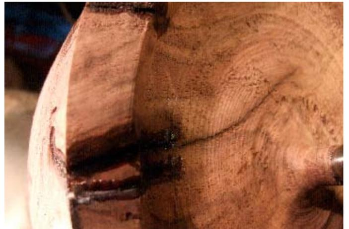
Since there was still a lot of wood to be turned away, and I wanted safety and stability as this vessel spun at 500 RPM, I squirted a copious amount of superglue in all the voids and cracks. The surface staining would all disappear as the wood was turned. Fig. 3 shows this process and you can surely see the results.
