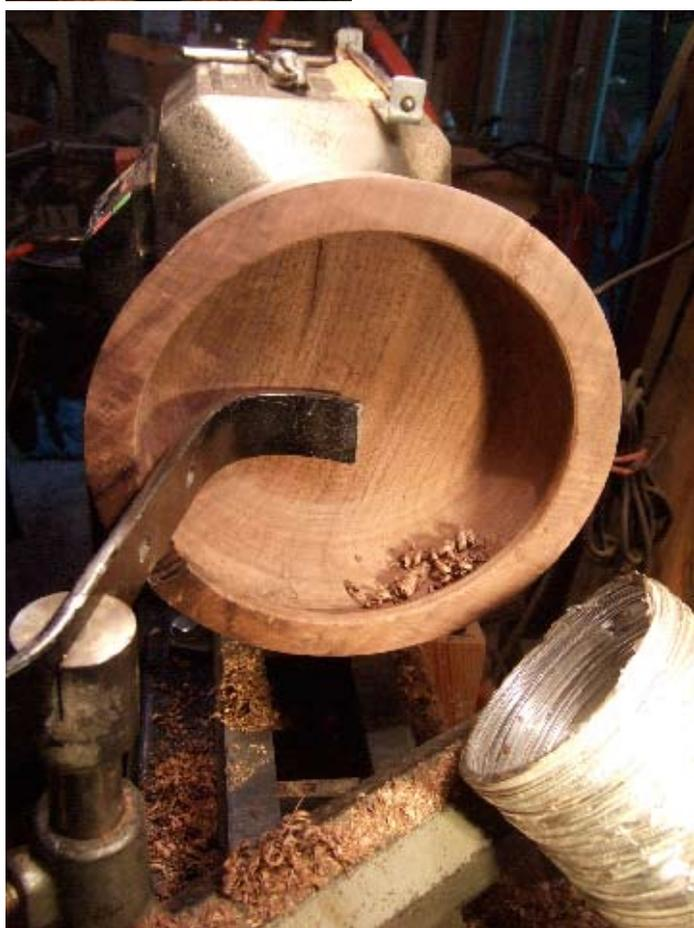
Fig. 12. The dark glue staining will eventually disappear into the interior's finish.
