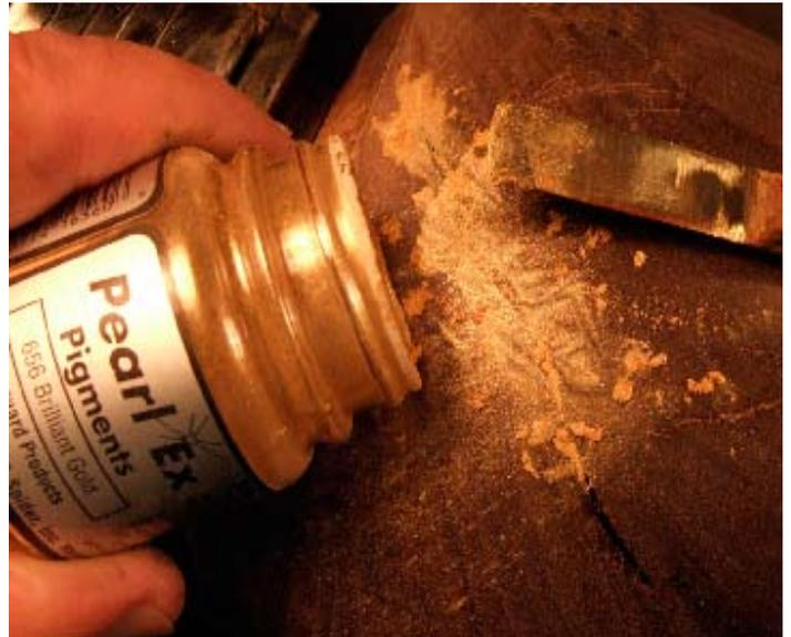
It is OK to smear a little excess onto (and into) wood adjacent to the cracks as later sanding will remove all but what is down inside the crack.
