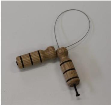
**6. Burning Wires.** Wire burned lines can often add a decorative touch. It is fast, easy, predictable, and economical. Materials to make a burning wire consist of a 1" x 1" x 6" piece of hardwood, two 1" drywall screws, and a 14" piece of guitar string. Guitar players often replace the strings and old strings work fine. Details can be seen in American Woodturner Magazine, August 2015, vol 30, no 4, on Page 28
