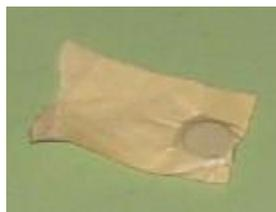
**12. Metal Detector.** Place a 1/2" rare earth magnet in about a 3" length of masking tape. Then just hold the end of the tape and drag the magnetic end over the surface and you will feel right away if there is a nail or screw in there.
