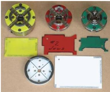
**2. Chuck Templates.** Lathe chucks have removable jaws to incorporate many different sized objects. They can compress over a tenon or expand into a recess. Often when turning an object, the size of the tenon or recess required has to be quickly known. Detailed plans, material list, and step-by-step instructions on how to build my version of Color-Coded Chuck Templates can be seen in Woodturning Design Magazine, Issue #24, Winter 2010, on Page 76.
