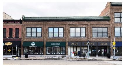
Figure 139: Example of appropriate contemporary window configuration and double-hung operation style at the second floor, but inappropriate fake muntins have been added to simulate a six-over-six double-hung window, not in the district.
