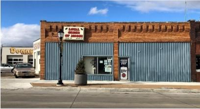
Figure 96: Example of inappropriate contemporary infill at a historic storefront with metal siding not in the district.
