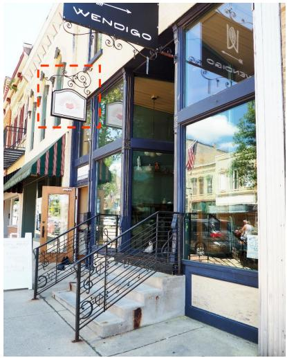
Figure 75: Example of an appropriate contemporary horizontal projecting sign anchored into the masonry mortar joints in the district.
