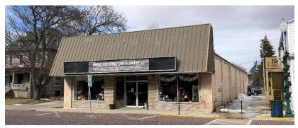
Figure 111: Example of a substantial inappropriate storefront alteration not in the district. The original brick facade and storefront have been obscured with a contemporary faux roof with a wide overhang to serve as a canopy.
