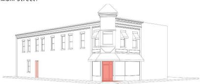
Figure 168: Illustration of a historic corner building in the district. New construction should include storefront entrances that are centered or offset to maintain the existing entrance patterns in the district and the location of the entrance to the upper floors at a primary façade.
