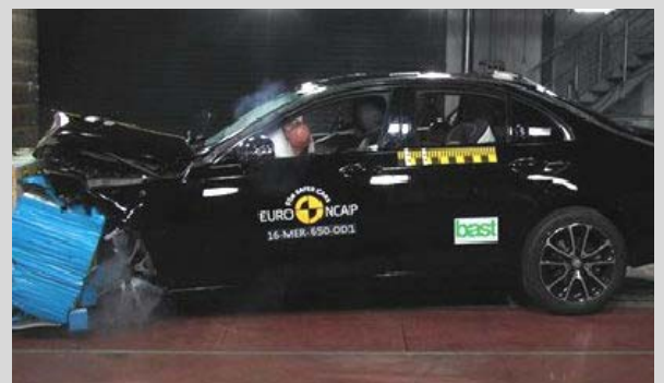
Frontal offset test at 64km/h
