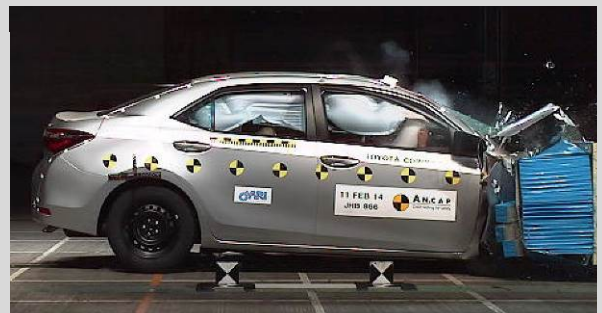
Frontal offset test at 64km/h
