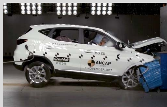
Frontal offset test at 64km/h
