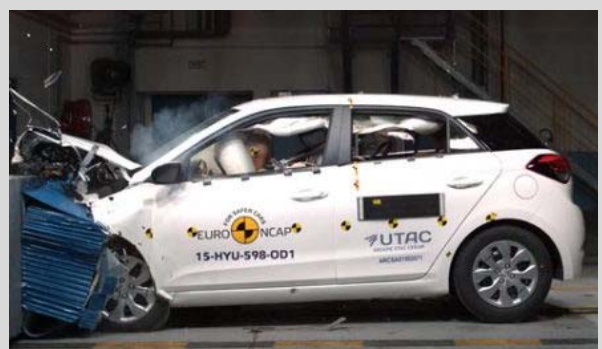
Frontal offset test at 64km/h
