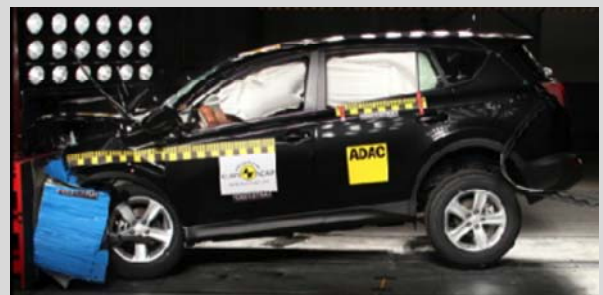
Frontal offset test at 64km/h
