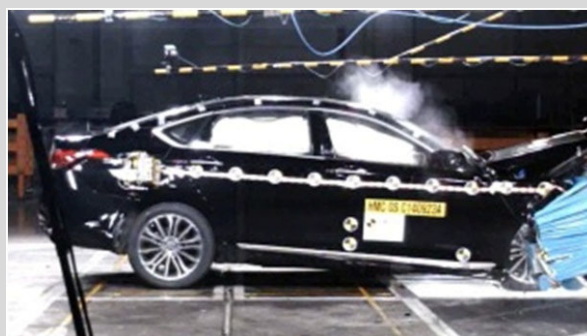
Frontal offset test at 64km/h
