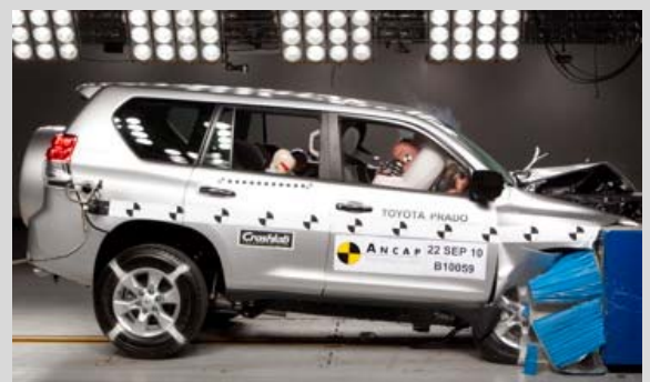
Frontal offset test at 64km/h
