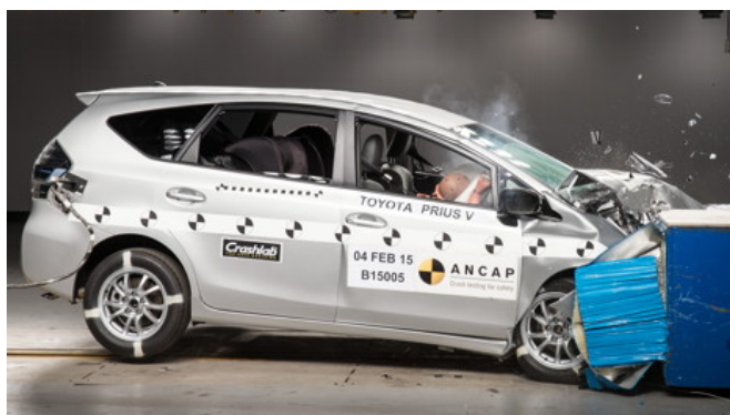
Frontal offset test at 64km/h
