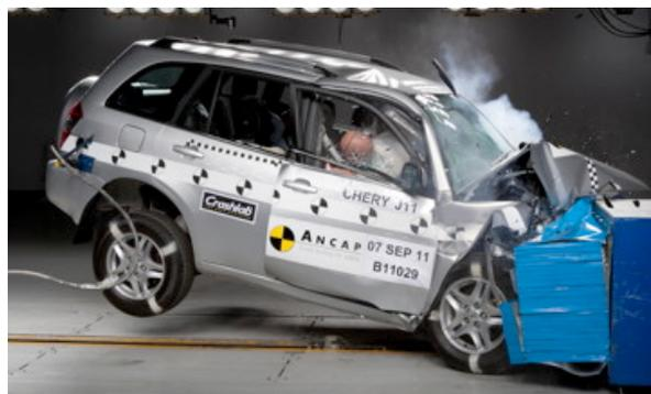
Offset crash test at 64km/h
