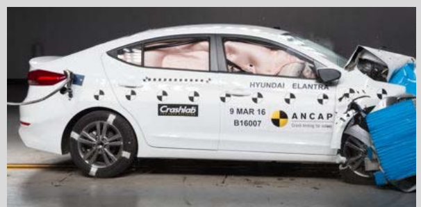
Frontal offset test at 64km/h (Hyundai Elantra)
