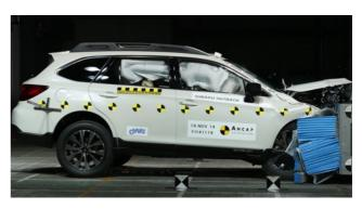
Frontal offset test at 64 km/h
