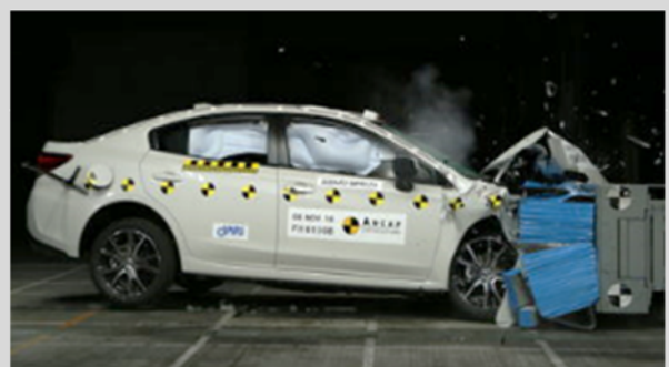
Frontal offset test at 64km/h
