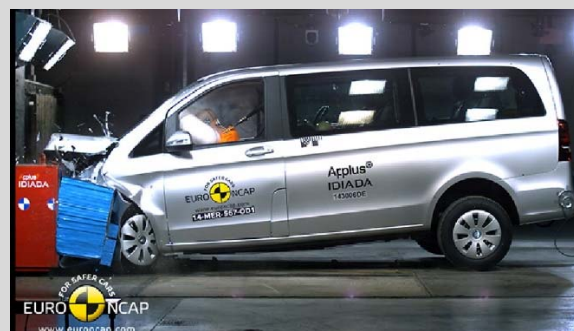
Frontal offset test at 56km/h (Mercedes-Benz V-Class)
