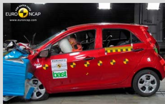
Frontal offset test at 64km/h
