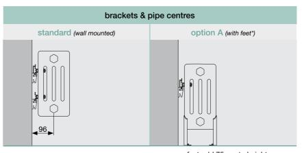
\* radiators over 20 sections in length have an extra pair of feet, for support, halfway along the length
