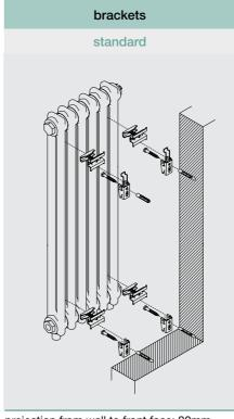
projection from wall to front face: 90mm (rail adds 80mm)
