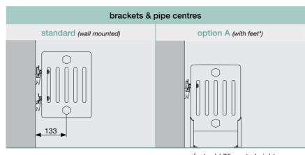
\* radiators over 20 sections in length have an extra pair of feet, for support, halfway along the length
