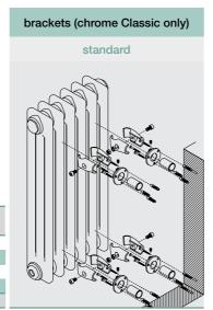
projection from wall to front face: 165mm to 175mm
