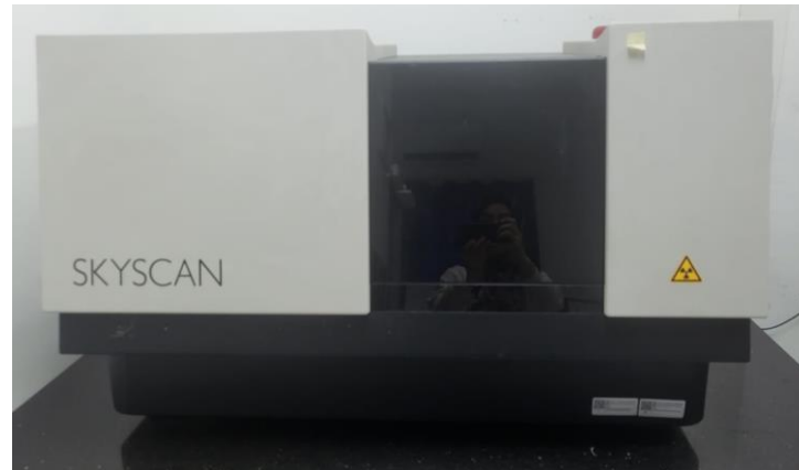
Gambar 2. Mesin Micro-CT di Lab Micro-CT scan FMIPA ITB
