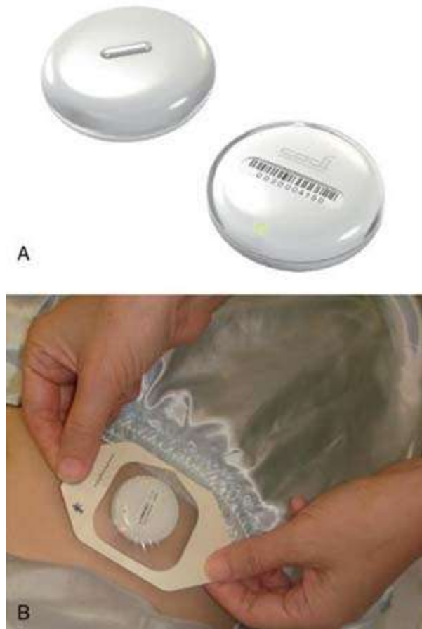
FIG. 17.2 (A) OR wireless thermometer. The disc has an elliptical cross section, and the sensing element consists of a metal strip located at the center of the skin-contact side. (B) ThermoSENSOR. The device has been placed over the first piece of hypoallergenic adhesive film dressing on the lower abdomen and is about to be secured to the lower abdomen by a second piece of the same dressing. Source: (From Ng, K., Wong, S., Lim, S., & Goh, Z. [2010]. Evaluation of the Cadi ThermoSENSOR wireless skin-contact thermometer against ear and axillary temperatures in children. Journal of Pediatric Nursing , 25[3], 177.)
