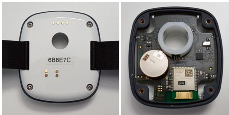
Fig. 12.1 Development version of a wearable device for measuring the skin parameters transepithelial water loss (TEWL) and electrodermal activity (EDA). Reproduced with permission by E트로plan GmbH, Endingen, Germany © 2024. All Rights Reserved
