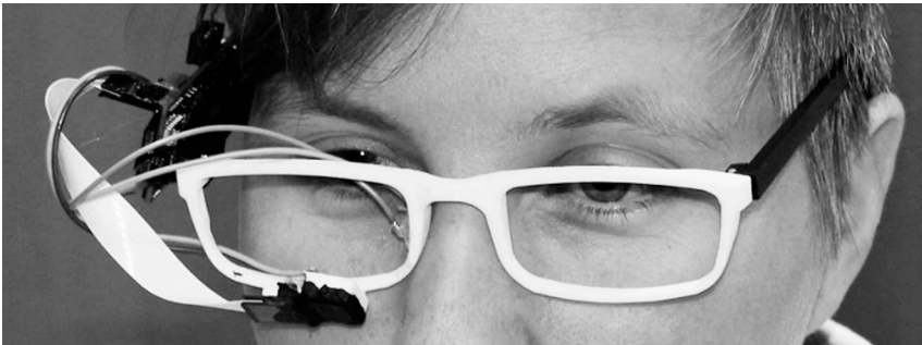
Figure 10a.1 Early Prototype of iShadow Computational Eyeglasses.
