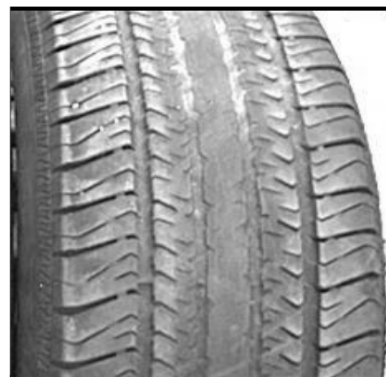
Fast Centerline Wear
