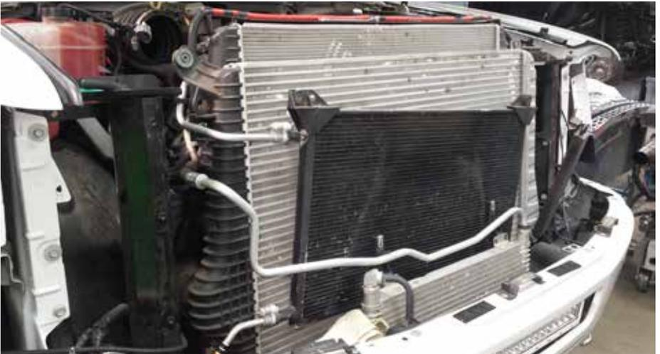
**23.** At this point the charge air cooler is ready for removal. Shown in **figure 9**
