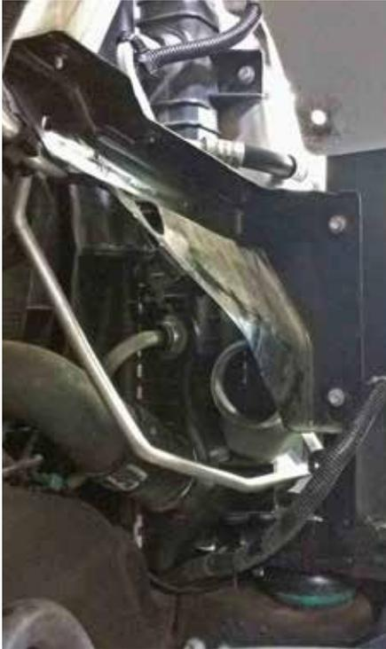
**18.** Pull the air conditioning condenser out of its lower mounts.
