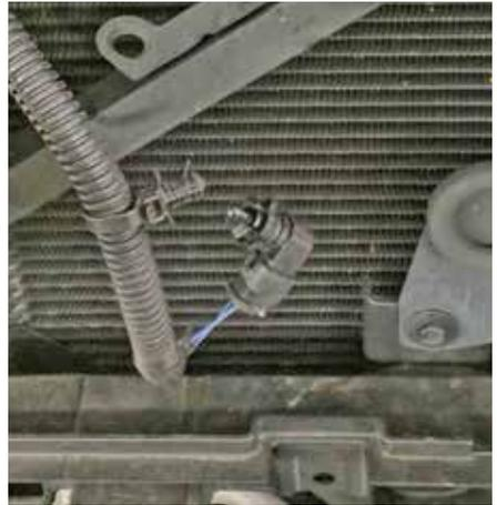
**14.** Mark the location of the hood latch, disconnect the hood latch electrical connector, then remove the hood latch from the latch support. The latch is held in place by three bolts. It is not necessary to remove the cable from the latch, just place the latch and cable assembly out of the way.
