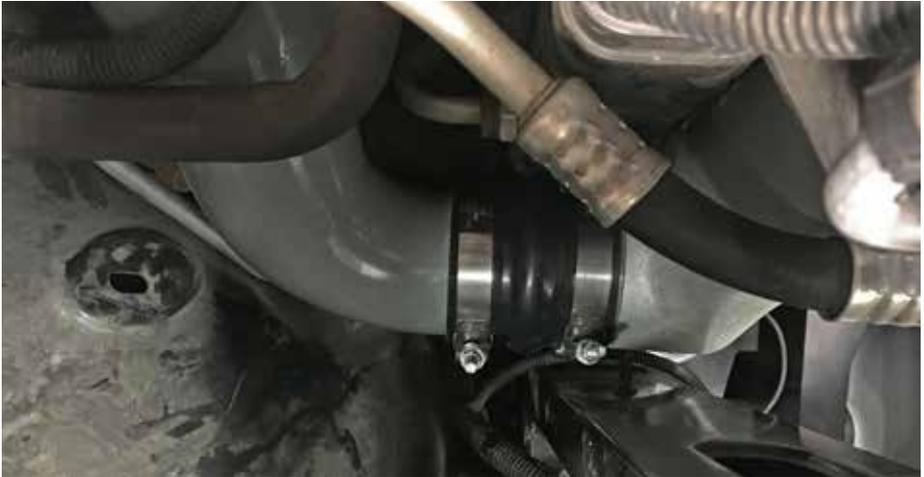
**37.** Install transition hose (Item #8) onto the throttle body inlet with clamps (Items #6 & 7) as shown in **figure 12**.
